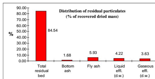
Figure 2: Fraction of the total amount of residual particulates recovered in different compartments of the unit rig.
