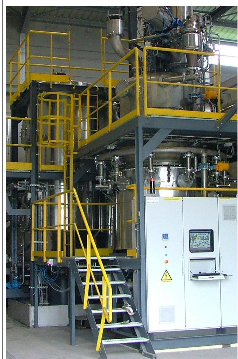
Figure 2: NOTAR® Gasifier powering CHP engine in Belgium
