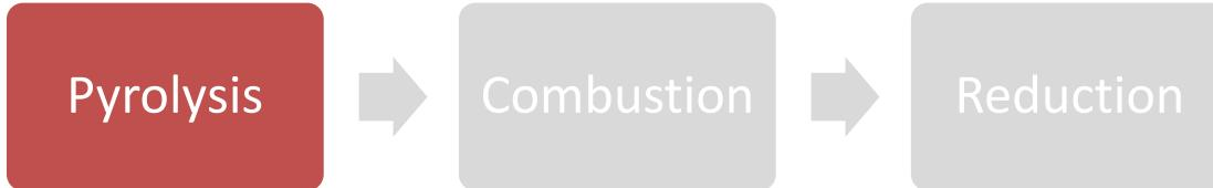
Heat is used to break down the fresh solid fuel into Charcoal (C) and into Pyrolysis gases (a mixture of light gases and tar (mainly primary & secondary tars, but almost no tertiary))).
